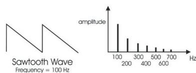
The sawtooth wave is the richest sounding of the four waves. It contains all of the harmonics, and has a bright, buzzy sound. Sawtooth waves are ideal for brass and string sounds, bass sounds and rich accompaniments.
