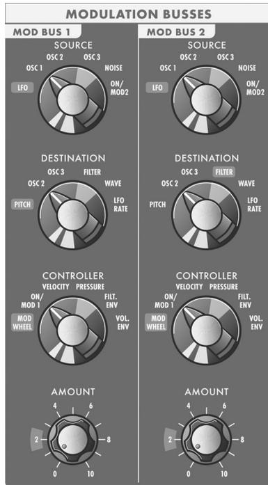
The Modulation Busses allow you to select a variety of modulation sources, destinations, modulation controllers, and amounts. The two Mod Busses are labeled MOD BUS 1 and MOD BUS 2, and are identical in function. The control of each mod buss is selectable instead of being tied to a particular controller, and six controller options are available.
