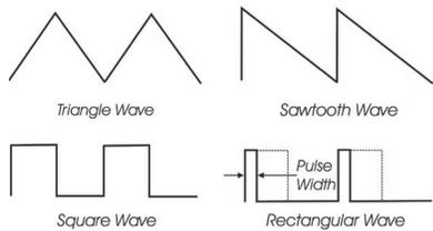
interesting timbral changes. By limiting the modulation between the square and rectangular waveform, you can get pulse width modulation (PWM). Although the waveforms can be set from the front panel individually for each oscillator, modulation through the Mod Busses affects all three waveforms simultaneously. When using modulation, it is possible to make the width of the rectangular wave so skinny that it becomes silent.
