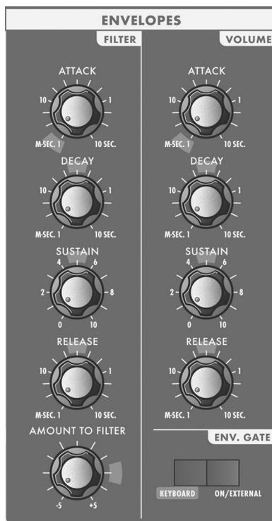
When triggered, EG's produce a time-varying control voltage that has a specific start, middle and end profile. The four parameters that define this profile are Attack, Decay, Sustain and Release, sometimes abbreviated as ADSR.
