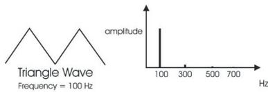
Like the square wave, the triangle wave only contains odd harmonics, but the levels of the harmonics in a triangle wave are much less. The triangle wave has a soft, slightly buzzy sound that is suitable for high-pitched leads (like a flute) or adding a beefy sub-bass to bass sounds.
