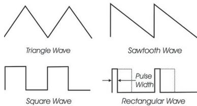
interesting timbral changes. By limiting the modulation between the square and rectangular waveform, you can get pulse width modulation (PWM). Although the waveforms can be set from the front panel individually for each oscillator, modulation through the Mod Busses affects all three waveforms simultaneously. When using modulation, it is possible to make the width of the rectangular wave so skinny that it becomes silent.
