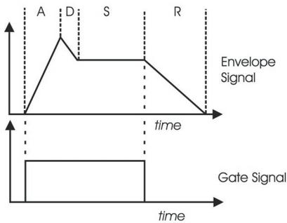
The second auxiliary component is the Envelope Generator, or EG. The EG makes no sound by itself. Rather, it creates a time-varying control voltage that is typically used to control the gain of the amplifier, or the cutoff frequency of the filter. Many synthesizers, including the Voyager, provide several EG's for independent envelope control of the amplifier and filter circuits.
