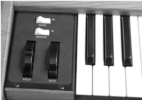
The Voyager OS has a 44-note keyboard (3½ octaves, F to C), just like the original Minimoog. The Voyager's keyboard produces velocity and aftertouch (pressure) voltages monophonically. These voltages can be used as modulation control signals through the Modulation Busses, or as external control signals when the Voyager is connected to the optional VX-351 CV Expander.
