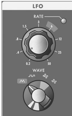
For the Sample and Hold circuit, the LFO's square wave is used as the S&H Trigger input, while the Voyager's Noise source is used for the S&H Input signal. For each positive-going cycle of the LFO square wave, the voltage at the input of the S&H circuit is sampled and held until the next cycle. Since the sample source is Noise (a random signal), the voltage that appears at the output of the S&H circuit is a random voltage that changes in time with the LFO.
