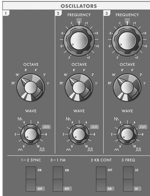
Oscillator 1 performs as a master oscillator to which Oscillator 2 and 3 are tuned. The timbres of the oscillators are adjusted by their variable Waveform controls. In addition, there are switches for Oscillator 2 sync to Oscillator 1; linear frequency modulation of Oscillator 1 by Oscillator 3; Oscillator 3 keyboard control ON/OFF; and Oscillator 3 Lo or Hi frequency range.
