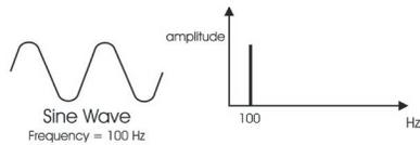
The sine wave is the purest waveform of them all. It has no harmonics, so it produces a very pure tone. Because of this, sine waves generally aren't used as primary audio signals, but are often used to reinforce or enhance other waves. They are also used as modulation sources.
